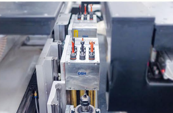
底部双钻包，每个钻包含9个垂直钻 Two Bottom drill banks both with 9 vertical drills
