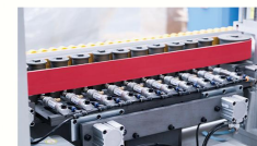
皮带压贴 Belt pressure zone
